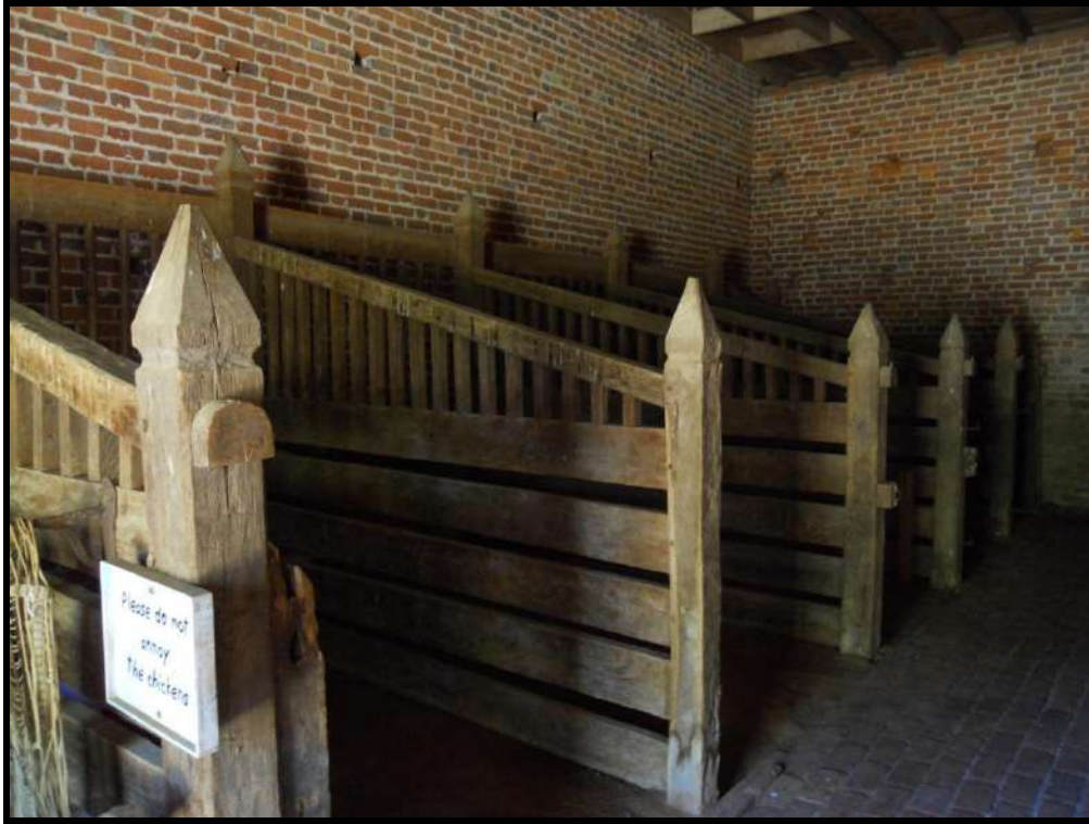
Figure 5 shows the standing stalls at Stratford Hall. The floors of the stalls are clay, while the aisle is paved in brick.
