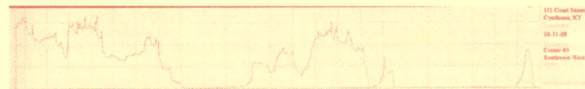
Results of a resistance drill reading. The low spots indicate decay.
