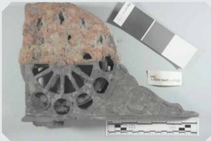
Cast-iron pulley halfway cleaned, Miriam McCue '16
